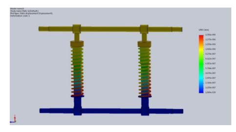
Figure 3 Force analysis with minimum load 200 Kg  $\,$
