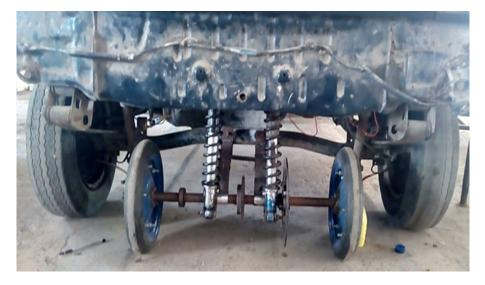
Figure 1 Sub wheel assembly
